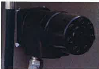
Direct drive motor drives 6" auger
