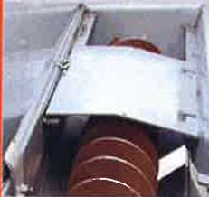
Anti-flow plate prevents material free flow and helps minimize material waste.
