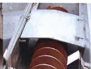
Anti-flow plate helps prevent free-flow of material
