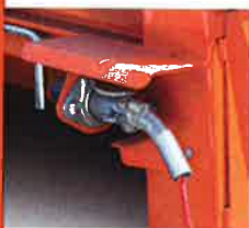
Patent pending Electric Interlock System disables auger when cover is opened.
